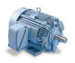
IP23, "Open Drip Proof" motors in Cast Iron frames enable higher powers to be accommodated in smaller frame sizes where IP55 protection is not required. These are generally used in compressors or enclosed air handling units. Various mounting options are available.
