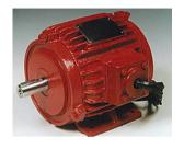
A wide range of Guardian "Smoke Spill" LV motors are available in pad mount format from UK Stock. These motors are rated at 300 °C for up to 2 hours and have been specified by a number of fan manufacturers. Other temperature classes and mounting arrangements are available.
