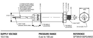
1/8 in - 27 NPT 0,609 m (2 ft) 4-Conductor shielded pairs 1.0 Vdc to 5.0 Vdc Output
